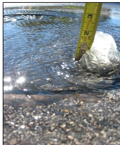
Figure 3: Manhole pick hole measurement
