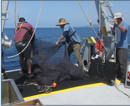
A trawl net is used to collect fish and large invertebrates from the ocean floor to conduct marine population assessments and fish tissue contaminant analysis.
