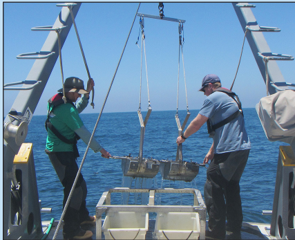
A grab sampler is used to collect sediment and small invertebrates from the ocean floor to conduct sediment contaminant analysis, sediment toxicity testing, and marine population assessments.
